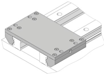
3. Slide the carriage onto the rails and set approximately the correct sliding resistance via the adjusting set screw. The exact setting is made later.
