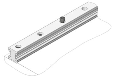
4. Screw the rail from the center outwards alternately.
