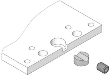
1. To mount the roller shoes, you first need the connecting plate with the adapter piece and the adjusting screw.
