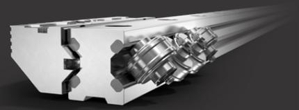
Franke aluminum linear systems have base bodies made of high-strength, anodized aluminum. Depending on the type, the rollers with needle or ball bearings are made of rolling bearing steel. Plastic end plates house felt wipers that keep the guide system clean.
