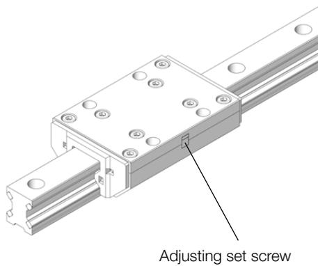
1. Remove the wipers from the cassette or roller blocks (see chapter 8.2). Slide the cassette or roller carriage on the rail.
